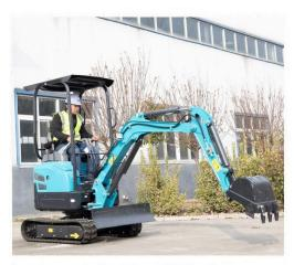
The TE-18S model bagger adopts Kubota D902 diesel engine, meets Euro V and EPA4 emission standards, meets environmental protection requirements, Low noise, Kubota engine parts are universal.
