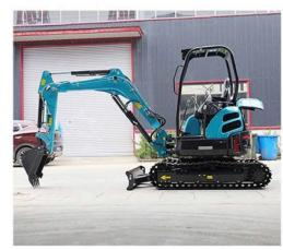
TE-35S small excavator is equipped with the Japanese Yanmar 3TNV88 three-cylinder water-cooled engine, which has strong power and good water-cooling heat dissipation effect.
